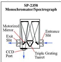
Figure 4. Includes dual exit ports; one exit slit and one sliding CCD adapter with motorized mirror for selection.
